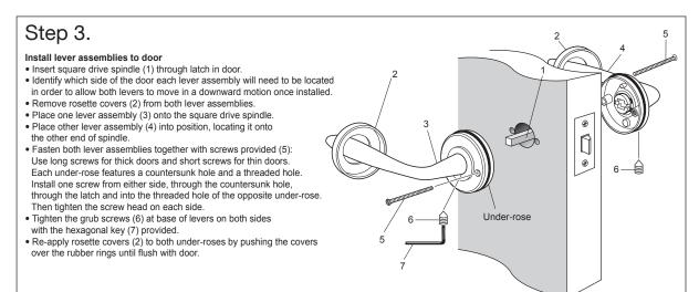
Carefully follow these instructions when installing. Screws to be tightened to a recommended 2.5Nm torque.
